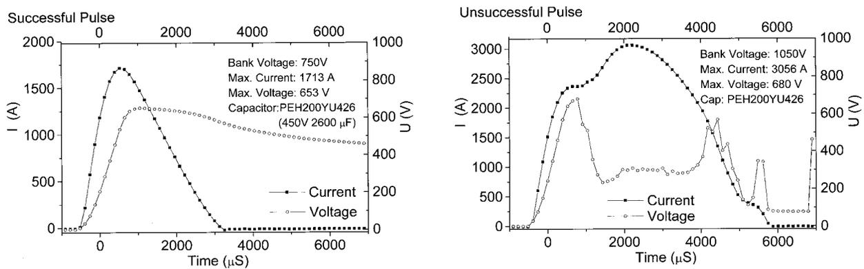
Figure 7. Successful and unsuccessful transient pulses on the same capacitor.
