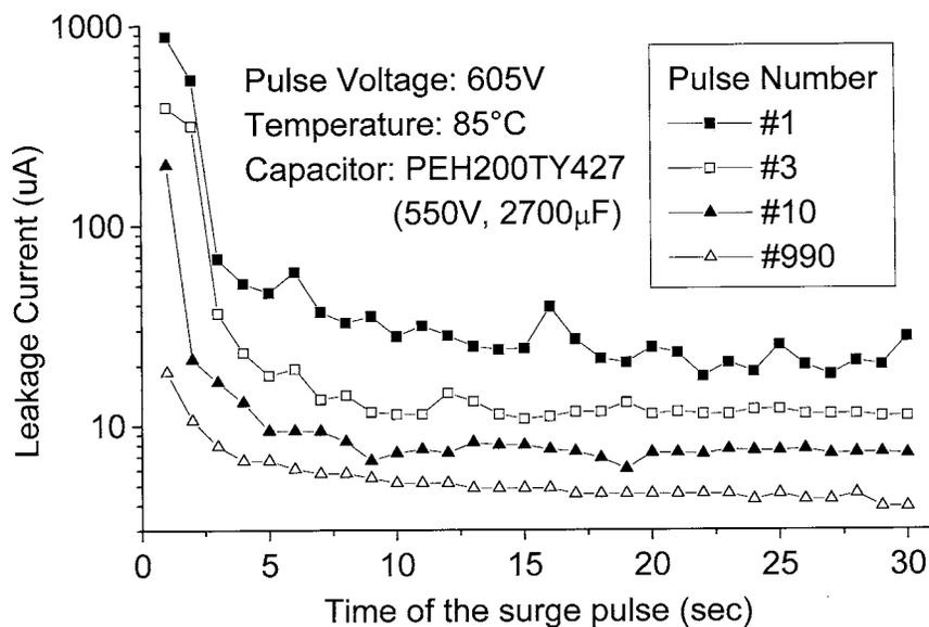
Figure 6. Leakage current behavior during surge pulses.
