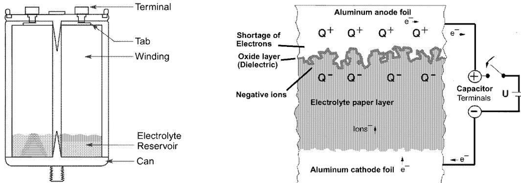
Figure 1. Construction of a typical screw terminal capacitor made by Evox Rifa.
