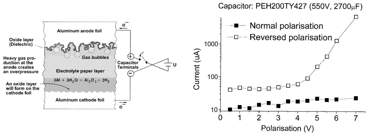
Figure 2. Reversed voltage operation.
