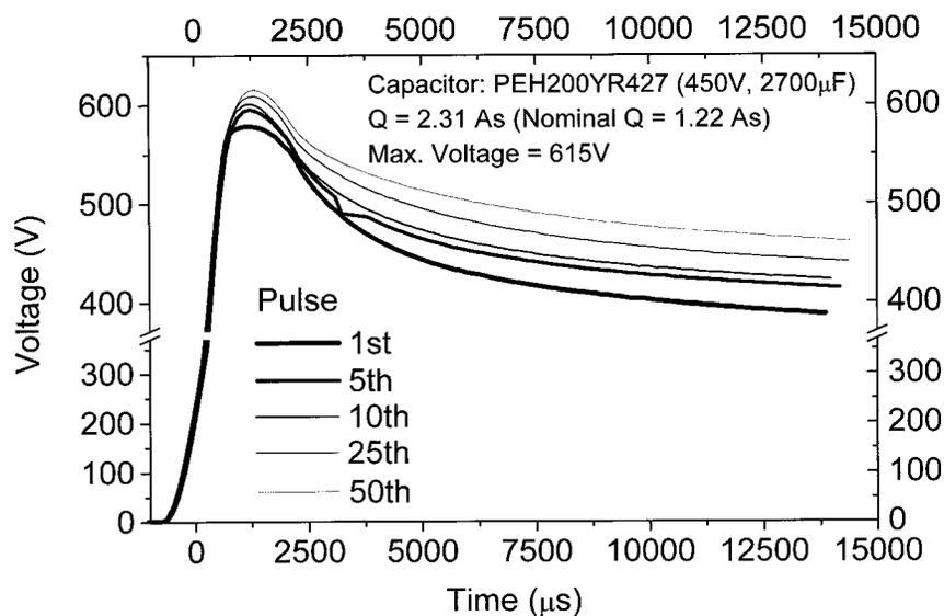
Figure 9. Cumulating charge in a double-load pulsing test.
