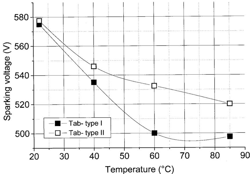
*Figure 5. Effect of temperature on the behavior of different types of tabs. Type II could be used for 500V capacitors with the given electrolyte, while type I is limited to 450V construction with the same electrolyte.*
