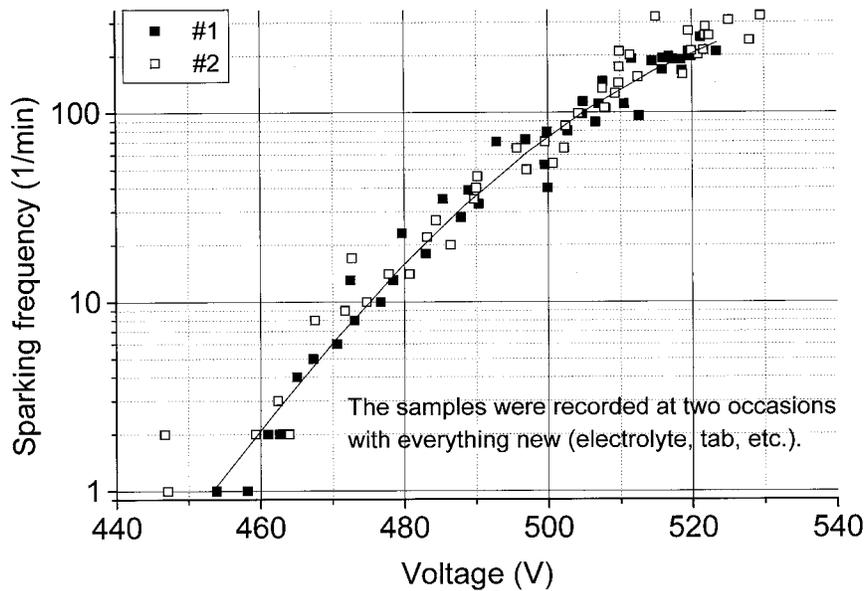
*Figure 4. Typical discharge characteristics at voltages near to and over the rated voltage for a new electrolyte formulation designed for 450V capacitors.*
