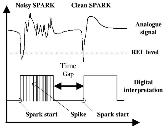
Figure 3. Schematic function of the sparking detector.
